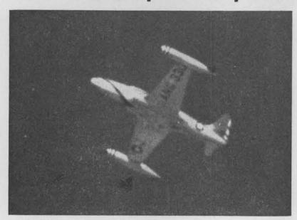
HIGH FLYING JET at a range of approximately 40,000 feet as photographed with the 24-inch telescope. This picture is indicative of the results that may be obtained when the tracking camera is used during ballistics tests. Exposure is 1/1000th second, no filter.
